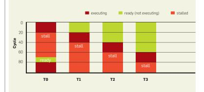
Figure B: Thread Execution on the example GPU core
