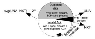
Figure 3: Ack Number Map. UNA is the lowest unacknowledged sequence number, NXT is the next sequence number that C will send. The 32-bit Ack field is cyclic.
