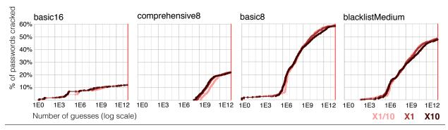
Figure 7: Varying the weighting of our passwords within the public training data among one-tenth (X1/10), equal weighting (X1), and ten times (X10) has little to no effect on the efficiency of cracking passwords. Results shown for four example conditions.
