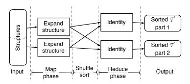
Figure 1: Distributed computation of the Weir-algorithm guess numbers using Hadoop. The framework splits the set of input structures and executes a map task for each subset. The map tasks emit tuples of the form  $\langle probability, pg, \Pi c_i \rangle$ . The framework sorts the the intermediate tuples using a *total ordering partitioner*. A reduce task, which in this case is the identity reducer, writes to storage a subset of the sorted tuples.
