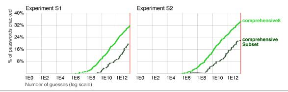
Figure 8: Passwords generated under the comprehensive8 condition proved significantly easier to guess than passwords that conform to the comprehensive8 requirements but are generated under other composition policies. In experiment S1, shown at left, the Weir calculator was trained with only public data; in experiment S2, shown at right, the Weir calculator was trained on a combination of our data and public data.
