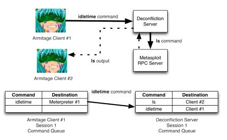
Figure 3: Meterpreter multiplexing in action
