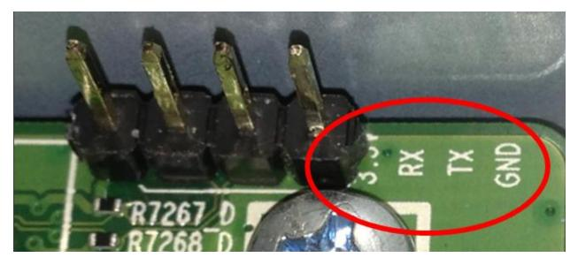
Figure 2 the four descriptions seen here are characteristic of UART
