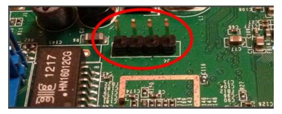
Figure 1 A common pin configuration for a UART interface
